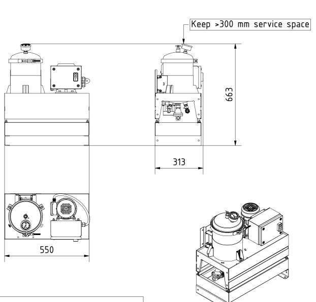
Single purifier unit. With safety shut off in tray. Absorbs water Removes soft and hard contaminants
